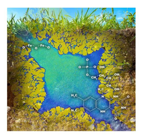
Integrated computational and experimental pore-scale reaction kinetics studies by a team of PNNL scientists revealed an approach to yield more accurate and scalable predictive models of biogeochemical interactions in soil. Shown above is the team's micromodel after reacting with reduced flavin mononucleotide at pH 7.0 for 21 hours. Blue indicates hematite coating; yellow indicates uncoated
