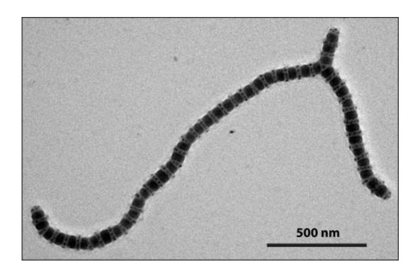
Transmission electron microscope image of a caterpillar micelle: Nanoparticles formed by self-assembly of terpolymers (A&#8211B&#8211C or A&#8211D&#8211C) are mixed so that they form a completely new superstructure resembling a caterpillar larva. Credit: photo/©: Müller Research Group
