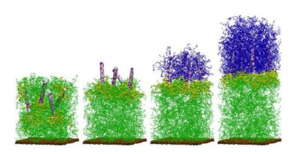
In the computer simulation, the composite is cut (far left) and the nanorods begin migration to the cut interface. In the third image, the polymerization from the rods surface and cross-linking initiates, culminating in the newly regrown gel (final image). Credit: University of Pittsburgh
