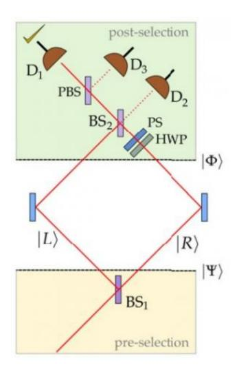
In the proposed experimental set-up, the quantum Cheshire Cat paradox is demonstrated when photons travel through the left arm of the interferometer while photon polarizations travel through the right arm. Some measurements disturb the photons and cause them to travel through the right arm with their polarizations, making the paradox seem to disappear. However, weak
