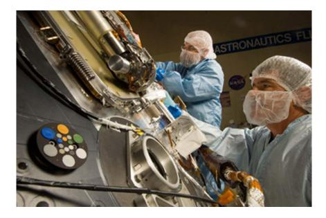
Lockheed Martin Space Systems technicians Jim Young (left) and Jack Farmerie (right) work on the science deck of NASA's Phoenix Mars Lander. The spacecraft was built in a clean room under NASA's planetary protection guidelines to prevent microbial life from being transported to Mars. Credit: NASA /JPL/UA/Lockheed Martin
