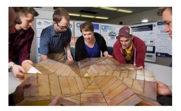
Mechanical engineering PhD student Shannon Zirbel and a team of students work on a solar array prototype that uses Origami.
