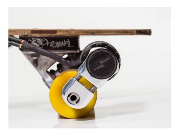
Purdue nuclear engineering student Joe Carabetta has invented a novel drivetrain "Kickr" that straps onto any long board, turning it into a fast, quiet, 20 mph, kickfree ride. Credit: Kickr
