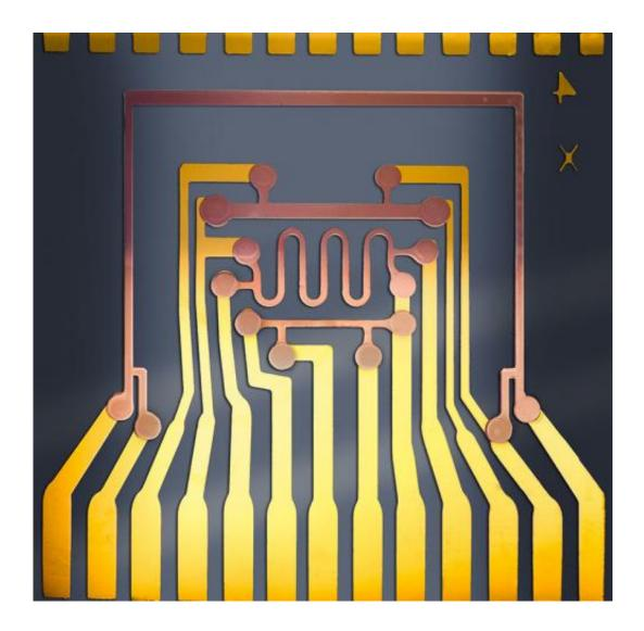
A close-up of the glass test cards for the e-Ca assembly used to detect moisture that seeps through film barriers. In the photo, the bright yellow lines are composed of calcium; the rust-colored traces are gold contacts. Credit: Dennis Schroeder
