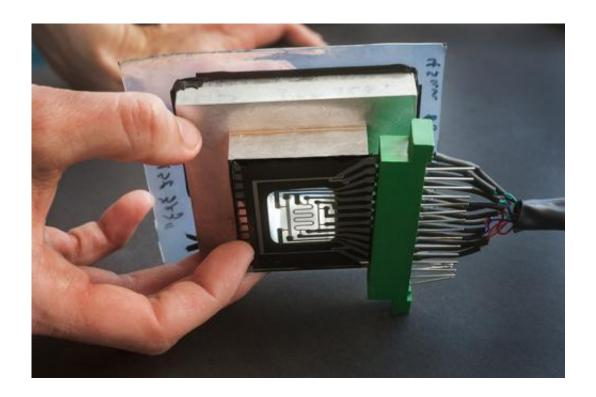
The e-Ca assembly is composed of a test card, a spacer, the barrier film, an edge seal to seal the components together, and a cable to connect the assembly to the measurement electronics. Module manufacturers want to be assured that any barriers they use will be able to pass the moisture-blocking test so they can focus on the rest of their module – and they want to make sure that anything they buy has passed rigorous quality control. Credit: Dennis Schroeder
