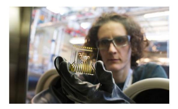
NREL scientist Arrelaine Dameron works with an Electrical Calcium Test (e-Ca) glass card in a glovebox. The test measures water permeating through the thin-film barriers that guard cell phones, TVs, OLEDs, and PV cells. Credit: Dennis Schroeder
