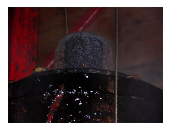
Gas bubbles in groundwater flowing from the open drill-stem casing during the drilling project. Very high helium concentrations were used to help identify the saline water's origin as Early Cretaceous North Atlantic sea water. Credit: Herbert Pierce
