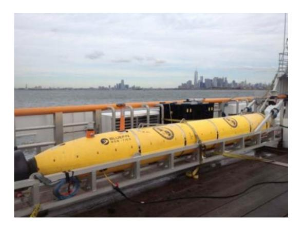
The NRL Reliant autonomous underwater vehicle (AUV), an advanced version of the Bluefin Robotics, Bluefin-21 vehicle, is the prototype for the new U.S. Navy Knifefish mine-hunter. The Reliant, shown here, outside New York City after completing a record setting endurance of 109 hours traveling nearly 315 miles. Credit: U.S. Naval Research Laboratory
