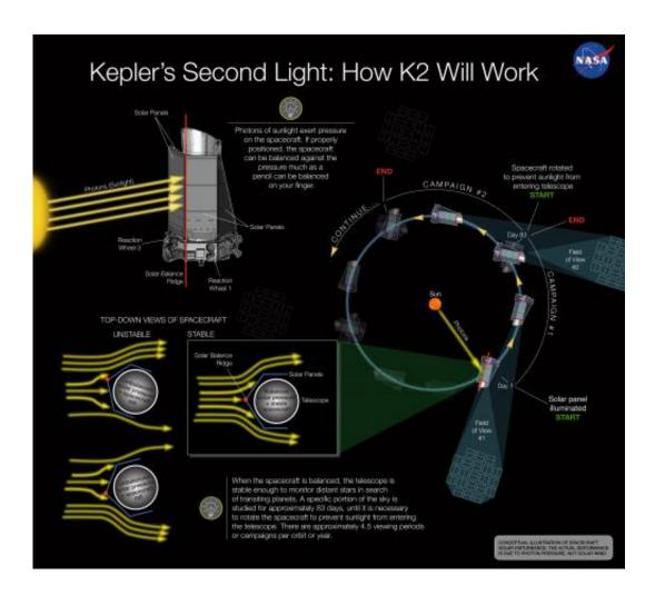
This conception illustration depicts how solar pressure can be used to balance NASA's Kepler spacecraft, keeping the telescope stable enough to continue searching for transiting planets around distant stars. Credit: NASA Ames/W Stenzel
