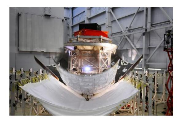
The three panel or fairings encapsulating a stand-in for Orion's service module successfully detach during a test Nov. 6, 2013 at Lockheed Martin's facility in Sunnyvale, Calif. Credit: Lockheed Martin
