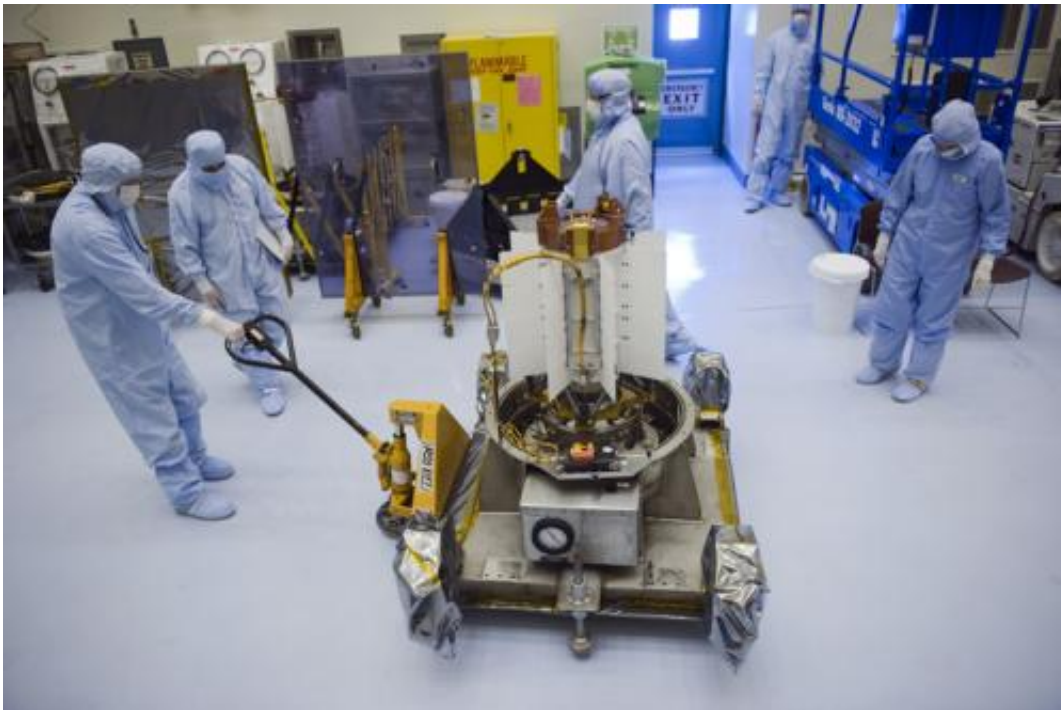
MSL's Pu-238 fueled MMRTG in the laboratory. Credit: NASA
