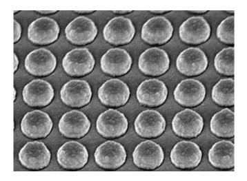
Altering the size and separation of these nanoscale mirrors changes the color of light that they reflect.
