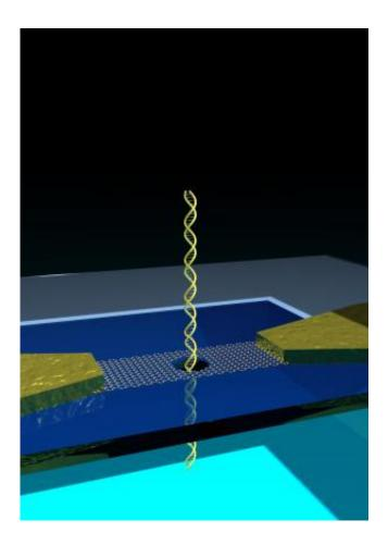
Many efforts over last decade have been directed towards development of single molecule sequencing based on solid state nanopores. Aleksandra Radenovic and co-workers have made a device composed of a graphene nanoribbon transistor built on top of a solid state nanopore. Direct electrical readout from the graphene transistors is used to detect DNA translocation events. Nanopore, DNA and the graphene nanoribbon are shown in this schematic (which is not to scale). Credit: EPFL
