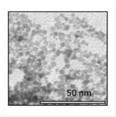
This is an image of the 3nm CeO2 nanoparticles taken with a transmission electron microscope. Credit: ESRF
