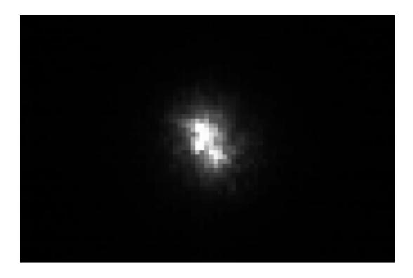
The first LADEE laser signal was acquired by ESA's Optical ground Station, Tenerife, Spain, at 06:36 GMT on 26 October 2013. The light beam from the Moon was transmitted at 1550 nm wavelength. Credit: ESA
