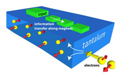
As current passes through a strip of tantalum, electrons with opposite spins separate. Researchers used the resulting polarization to create a nanomagnetic switch that could one day replace computer transistors. Credit: Debanjan Bhowmik, UC Berkeley
