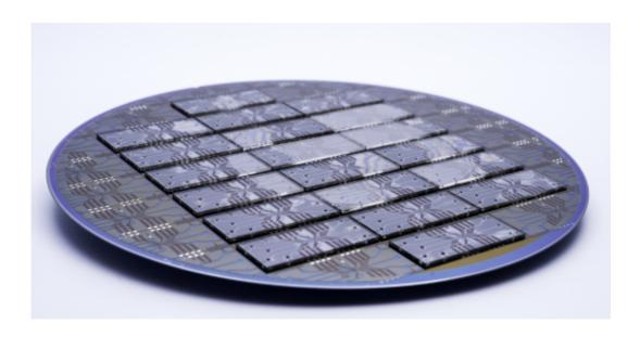
Cell sorter lab-on-chip, wafer processed at imec using JSR's novel PA.
