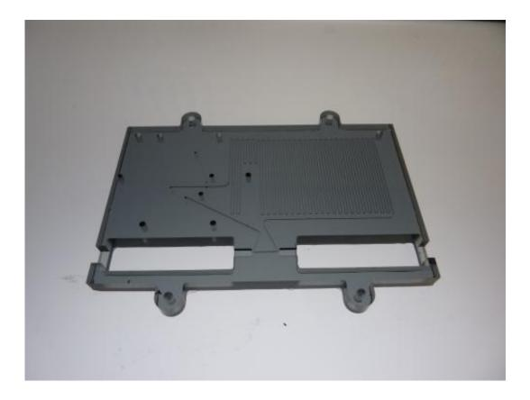
The image shows the microfluidic chip used in the pH micro sensor. Dimensions: 13 x 8 cm. Credit: National Oceanography Centre. Credit: National Oceanography Centre
