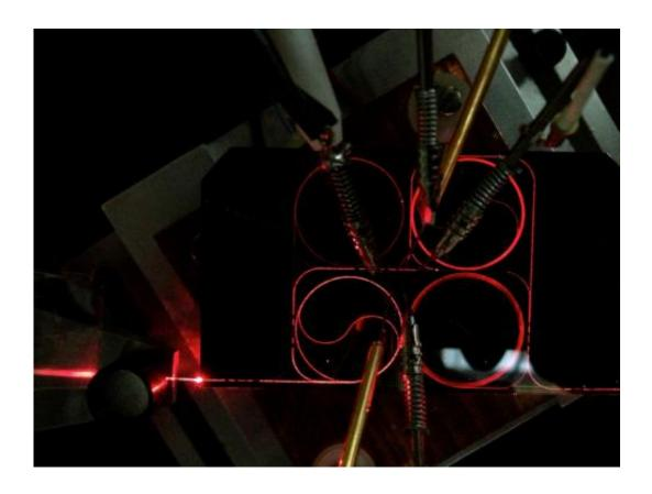
Ultra-low loss, true-time delay chip developed at the University of California, Santa Barbara with four different delay lines.
