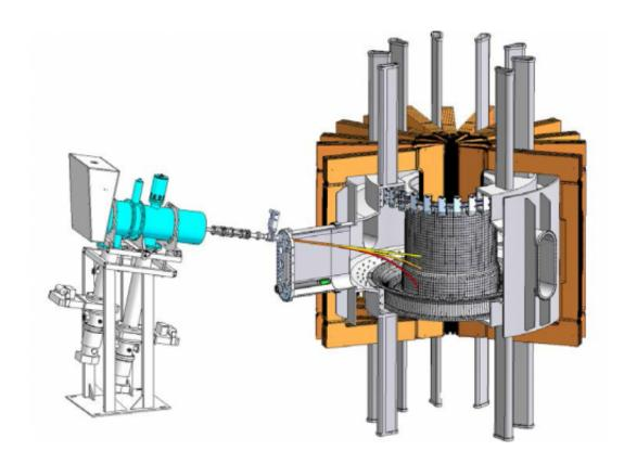
A small linear accelerator (left; cyan colored) injects a beam of energetic ions into the Alcator C-Mod tokamak (right). The ions are magnetically steered with tokamak magnets (copper colored) to different locations (yellow, orange, and red colored) on the wall. Analyzing the nuclear reaction products with small detectors (green colored) induced by the beam provides crucial information about the materials inside the device. Credit: Zach Hartwig
