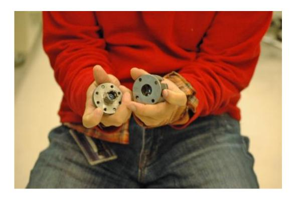
The diamonds are embedded in a steel casing that is used to apply extreme pressure on the rock samples. Studying how surface rocks change under high pressure and temperature helps researchers understand how rocks behave deep within the Earth's mantle. Credit: Kristen Hwang
