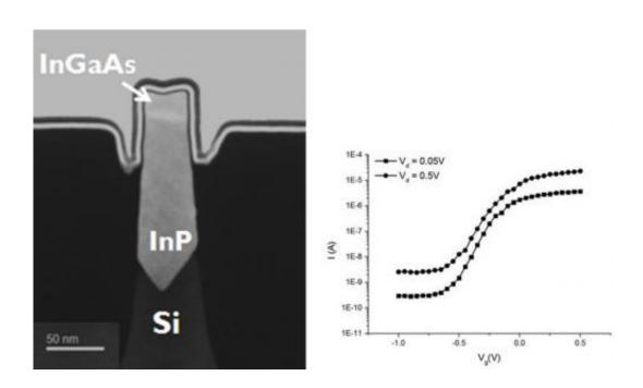
Imec, a leading nanoelectronics research center, announced today that it has successfully demonstrated the first III-V compound semiconductor FinFET devices integrated epitaxially on 300mm silicon wafers, through a unique silicon fin replacement process. The achievement illustrates progress toward 300mm and future 450mm high-volume wafer manufacturing of advanced heterogeneous CMOS devices,
