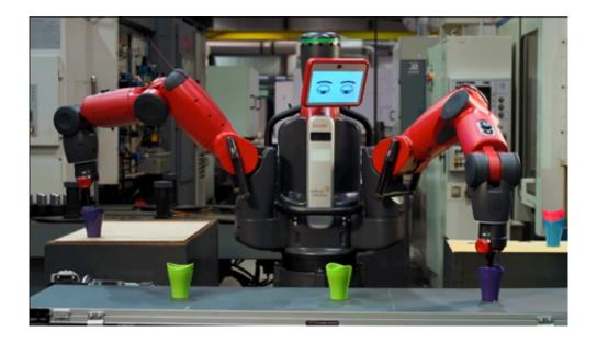
With multiple joints, a Baxter robot can move more flexibly than a human, but it would be hard for a human to decide how best to use those arms, so the robot is programmed to plan its own movements, then allow humans to make corrections.
