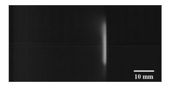
This is an image of lithium emission during experiments conducted on the Magnum-PSI device. Plasma streams toward the target from the left and impinges the sample indicated by the yellow dashed line. The lithium ablates into the plasma stream and forms a cloud in front of the target. Credit: M. Jaworski
