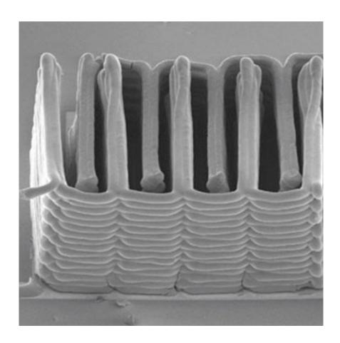
This image shows the interlaced stack of electrodes that were printed layer by layer to create the working anode and cathode of a microbattery. (SEM image courtesy of Jennifer A. Lewis.)
