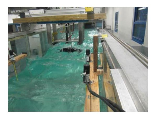
This image shows experimental measurement of the drag on a partially submerged waterbird in waves. Credit: FAU/K.von Ellenrieder
