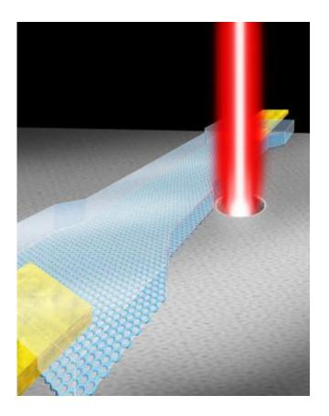
An illustration of an electron beam drilling a notch-shaped nanopore in a graphene nanoribbon.
