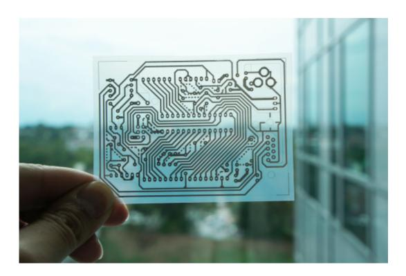
A single-sided wiring pattern for an Arduino micro controller was printed on a transparent sheet of coated PET film.
