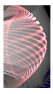
This is a typical structure of a peeling-ballooning mode in the DIII-D tokamak, calculated by ELITE. Credit: Philip Snyder
