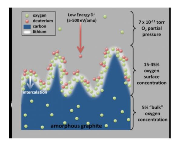
The lithium coating on graphite, which appears mountainous in this graphic done at microscopic scale, provides the perfect setting for oxygen to control the hot deuterium plasma. Credit: C.N. Taylor and J.P. Allain
