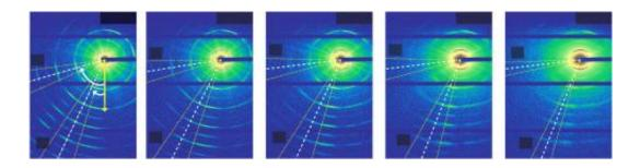
SAXS diffraction patterns generated at ALS beamline 7.3.3, shown for five points during mechanical testing of an Arapaima fish scale, reveal how lamellae in the scale rotate in response to an applied stress to resist fracturing.
