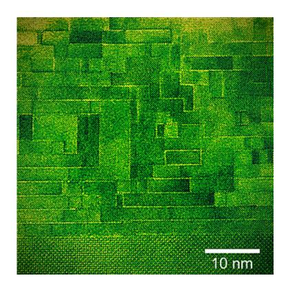
Not a brick wall. Electron microscope image of a cross section of the newly characterized tunable microwave dielectric clearly shows the thick layers of strontium titanate "bricks" separated by thin "mortar lines" of strontium oxide that help promote the largely defect-free growth of the bricks. Credit: TEM image courtesy David Mueller. Color added for clarity by Nathan Orloff.
