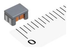
TDK Corporation presents a new series of common-mode chokes for automotive Ethernet that features the world's best common-mode noise suppression. Measuring in with a footprint of 4.5 mm x 3.2 mm and an insertion height of just 2.8 mm, the miniaturized ACT45L series is the world's smallest common-mode choke for automotive Ethernet and fulfills the standard's stiffest requirements. Mass production of the new common-mode choke starts in November 2013.
