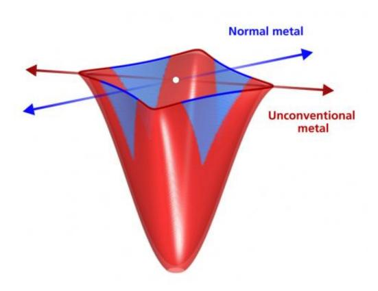
Electronic band structure of overdoped La1.77Sr0.23CuO4, shown schematically. The red and blue arrows indicate high-symmetry directions in momentum space. The figure illustrates how electrons along one high-symmetry direction (blue) behave as in a conventional metal but along another direction (red) they have unconventional behavior.
