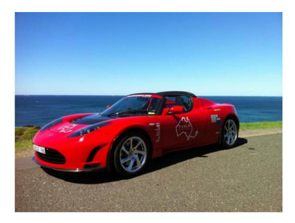
The 2011 Tesla Roadster Sports could hit 100 km/h in less than four seconds and be charged from a standard power point.
