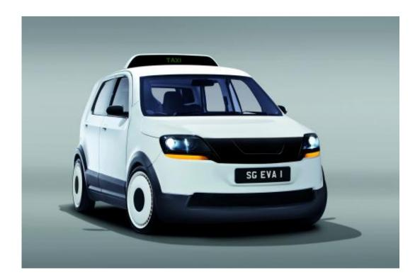
At the 43rd Tokyo Motor Show electric taxi "EVA" showcases a new super-fast charging system recharging the battery within 15 minutes, a range of 200 kilometers and an individual air conditioning. EVA has been developed at TUM CREATE, a joint research program by Technische Universitaet Muenchen and Nanyang Technological University. Credit: TUM CREATE
