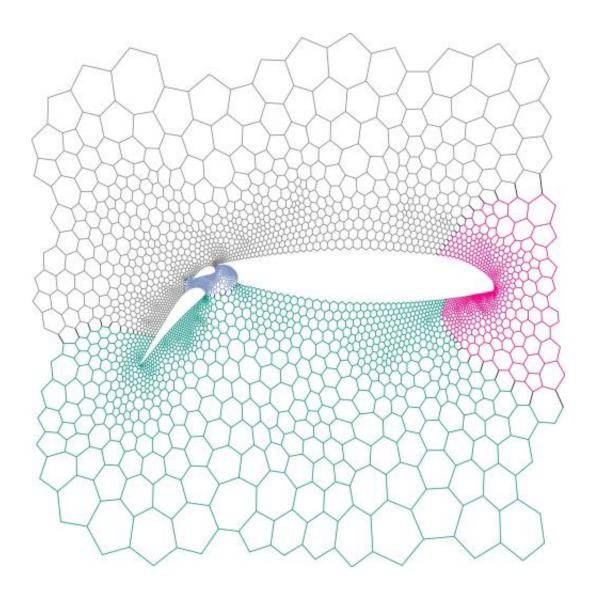
Graph to compute the air flow around an airplane wing: The four colors reflect the partitioning of the graph and, hence, the distribution of computation among four computers. Credit: Christian Schulz, KIT
