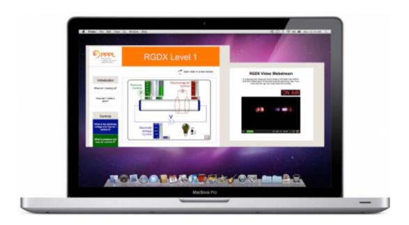
Remote users can operate a plasma experiment with a set of controls, shown on the left side of the screen, and watch the effect on the apparatus at PPPL using the web stream video, Credit: A. Dominguez and A. Zwicker
