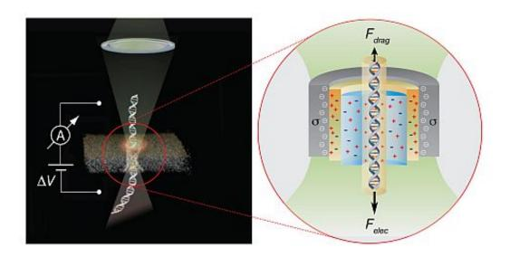
The Opto-electrical effect can be used to control the passage of DNA molecules through nanopore sensors, thereby leading to more accurate sensing and sequencing of individual DNA molecules.
