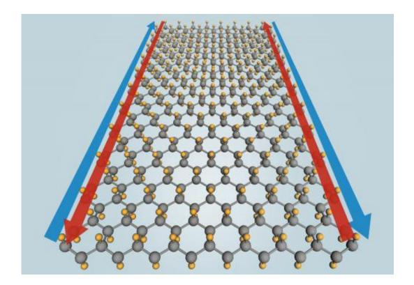
Adding fluorine atoms (yellow) to a single layer of tin atoms (gray) should allow a predicted new material, stanene, to conduct electricity perfectly along its edges (blue and red arrows) at temperatures up to 100 degrees Celsius. The first application for this stanene-fluorine combination could be in wiring that connects the many sections of a microprocessor, allowing electrons to flow as easily as cars on a freeway. Credit: Yong Xu/Tsinghua University; Greg Stewart/SLAC
