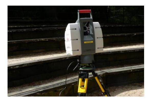
An example of a conventional lidar scanner that gauges depth by emitting laser light and measuring the time it takes for photons to rebound. MIT researchers developed a lidar-like system that can gauge depth by measuring only a single reflected photon. Credit: Wikipedia
