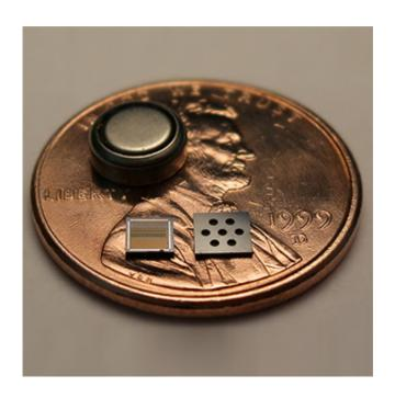
Researchers at Berkeley Engineering and UC Davis are developing a tiny chip that uses ultrasound waves to detect a slew of gestures in three dimensions. The technology, called Chirp, could eventually be used in everything from helmet cams to smart watches.
