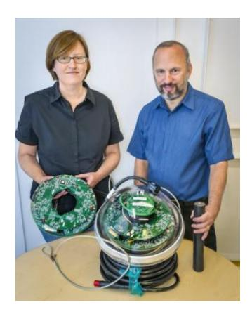
Pictured are Lisa Gerhardt and Spencer Klein with an IceCube Digital Optical Module (DOM). IceCube employs 5,160 DOMs to detect the Cherenkov radiation emitted by high-energy neutrino events in the ice. Credit: Roy Kaltschmidt, Berkeley Lab
