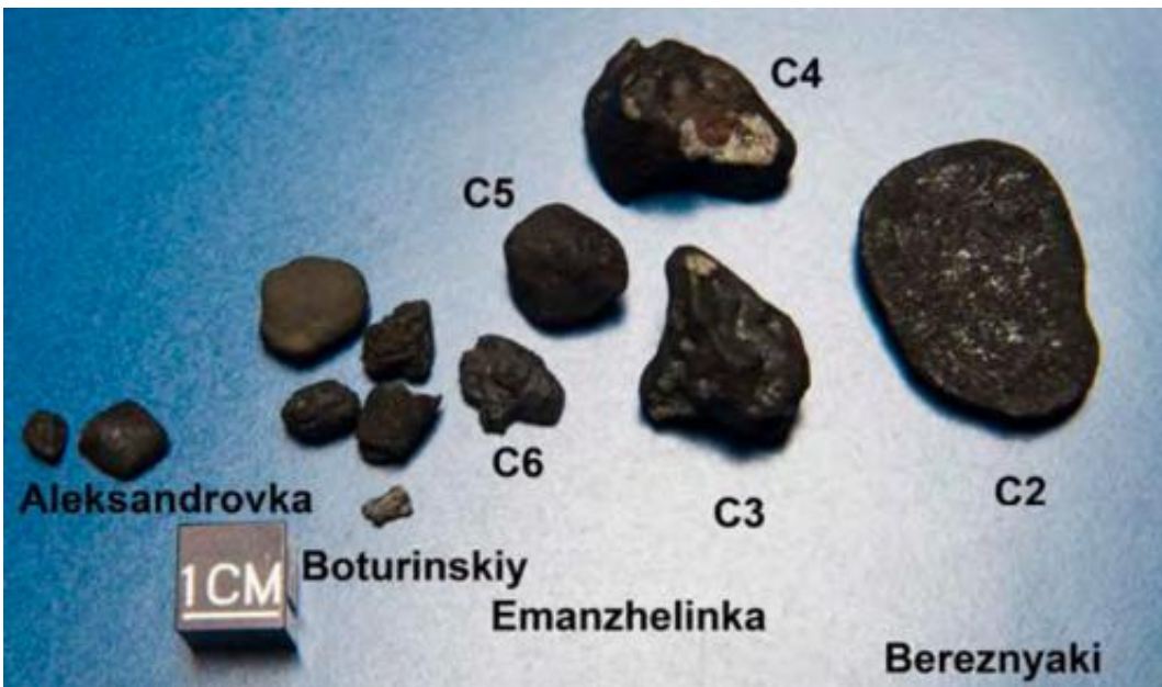
Fragments of Chelyabinsk (C2 - C6). C2 is an oriented meteorite; it travelled with its flat side forward. Its backside is shown. Credit: Science/AAAS
