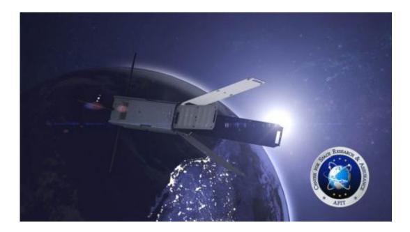
An artist rendering shows what the ALICE CubeSat will look like in space. Developed and built by the Air Force Institute of Technology, the micro-satellite will test the operation of carbon nanotubes as electron emitters in space. Credit: Air Force Institute of Technology
