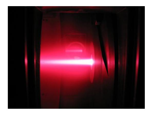
In the Pilot-PSI device researchers can expose materials to extreme conditions, such as those that will prevail at the wall of future fusion reactors. Credit: DIFFER.
