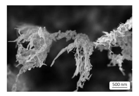
Even at a plasma bombardment that is 10,000 times more intense than the standard production method, carbon nanostructures such as these can develop. Credit: K.Bystrov / DIFFER.
