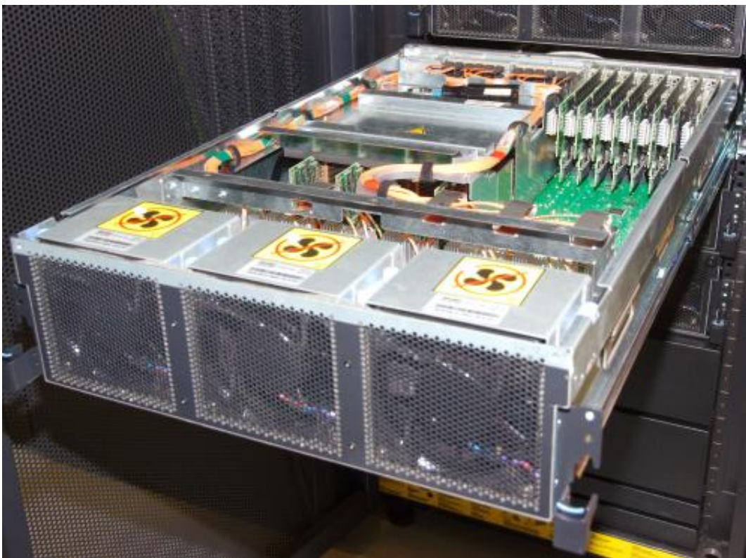
Drawer of the Blue Gene Active Storage system containing eight HS4 Cards (at the back right). In total, four of these units are incorporated into the system.
