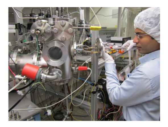
Clemson graduate student Githin Alapatt tests a silicon sample using the Copper Oxide Deposition System. Credit: Clemson University
